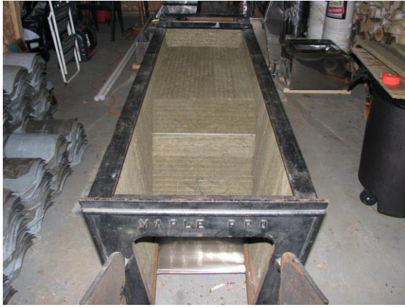
Insulation board laid out in the arch
